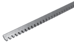
CRIS400 - COD. 162324 Rack in galvanized steel. 22x22x1000 mm to be welded, M4 (10pcs / pack)
